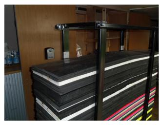
8 - Using mallet or block of wood, tap the foam from the back against the vertical bars on front of the jig
